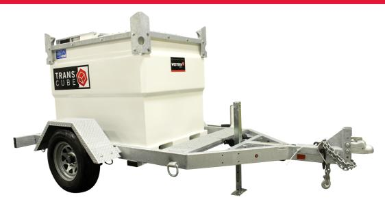
The TransCube Cab allows you to transport fuel easily on a jobsite. With a large lockable equipment cabinet and a double-walled design, the TransCube Cab is your safe and easy-to-use mobile refueler.
